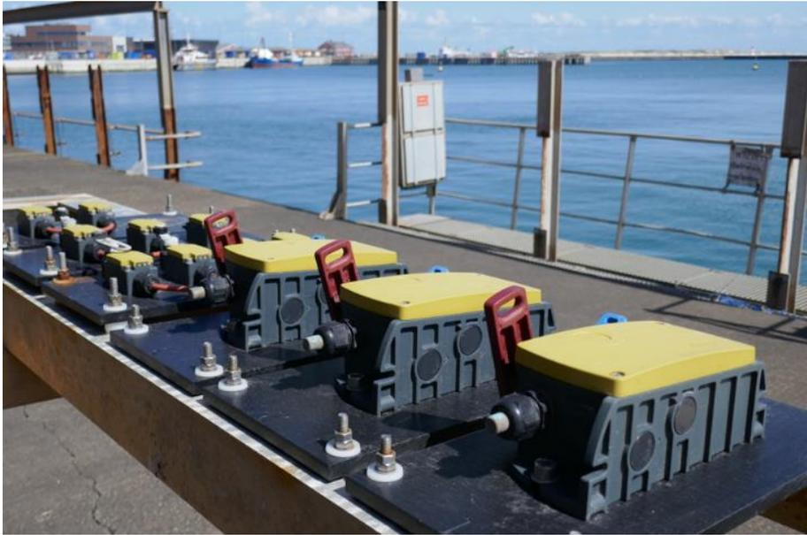
*Interim checks after seven months of outdoor exposure on the island of Helgoland: the emergency pull-wire switches are still fully functional*
