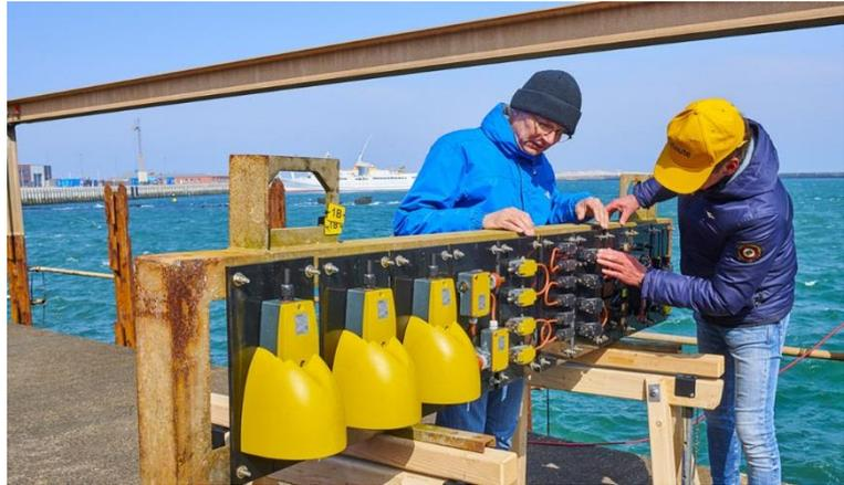
*More realistic than laboratory tests: in a one-year outdoor exposure test, "oil & gas" switches were tested on the North Sea island of Helgoland, some of them in tidal water. The photo shows the condition of selected switches at "half time".*
