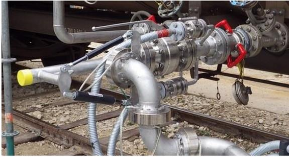
*The key components of these handling systems include the swivel joints of the loading arms, which are tightly sealed to prevent both gas and liquid leakage.*
