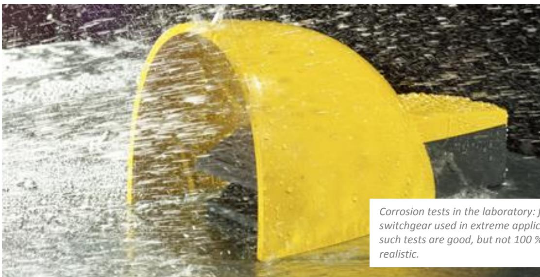
*Corrosion tests in the laboratory: for switchgear used in extreme applications, such tests are good, but not 100 % realistic.*
