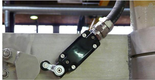
*The position of the loading arm is monitored using a position switch which must be suitable for extreme environments.*
