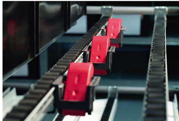
*Wireless sensors developed especially for eKanban racks manage the replenishment of materials in modern factories*
