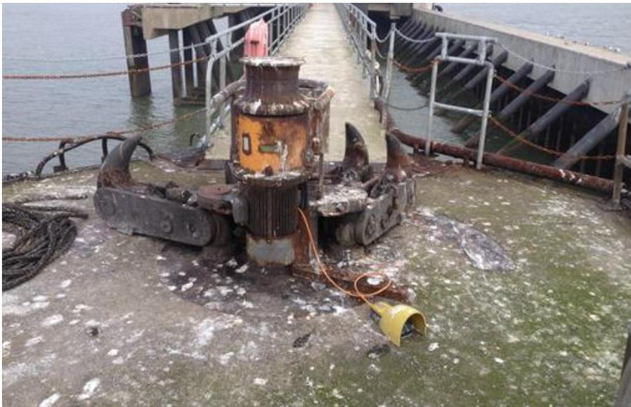
*This foot switch for actuating a winch on a mooring hook is continually exposed to saltwater, fouling and seagull droppings – and yet functions perfectly.*
