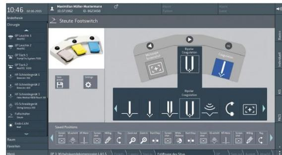
Fig. 3: The surgeon defines via touch screen or voice control which medical device is operated with the user interface
