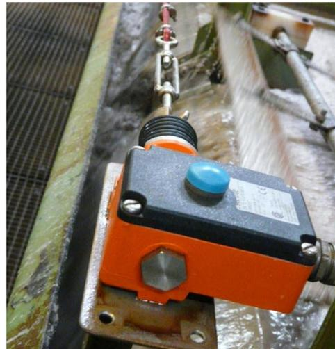
*The flotation systems are safeguarded using emergency pull-wire switches*
